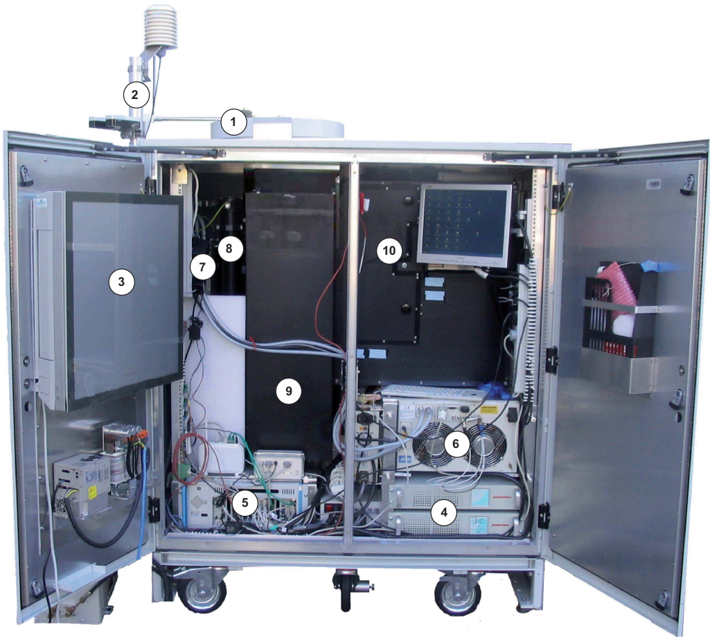
Figure 3.4: Cabinet with open doors showing the major parts of Polly XT . 1: roof cover, 2: sensors for outdoor temperature, air pressure, and rain, 3: air condition, 4: uninterruptible power supply, 5: computer with data acquisition, 6: laser power supply, 7: laser head, 8: beam expander, 9: receiver telescope, and 10: receiver with seven channels.
